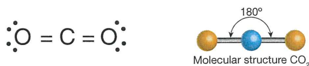
Figure 7.1 Carbon dioxide – Lewis electron dot structure and shape of the molecule.
